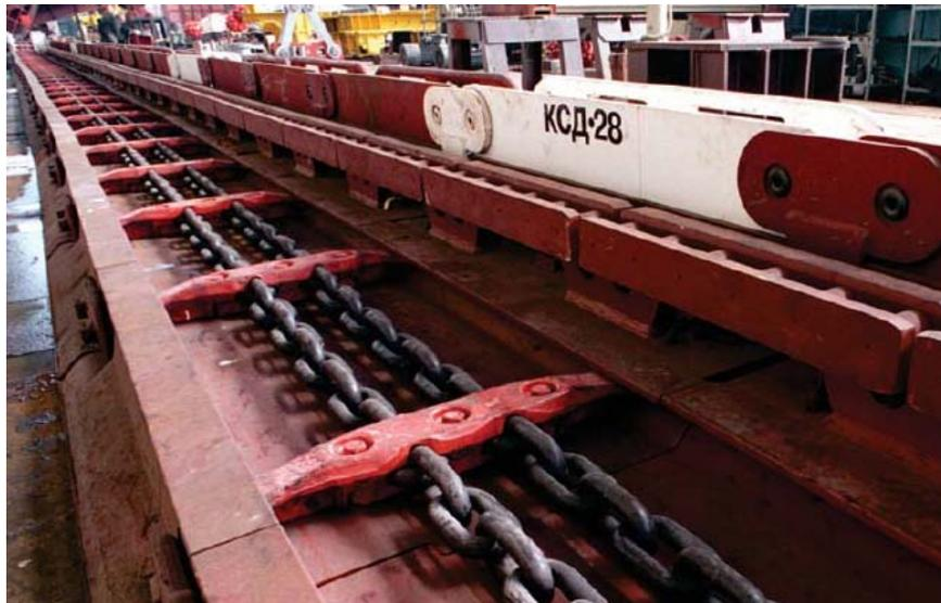
The conveyor is designed for coal transportation from highly-production (3000-8000 t/day) stopes with the length of 200-350m, working out the seams with the thickness of 1,4-2,4m and advancing to the strike with dip angles of up to 30°, as well as to the dip or the rise with angles of up to 10°, in mines, including those that are hazardous by gas and dust.
