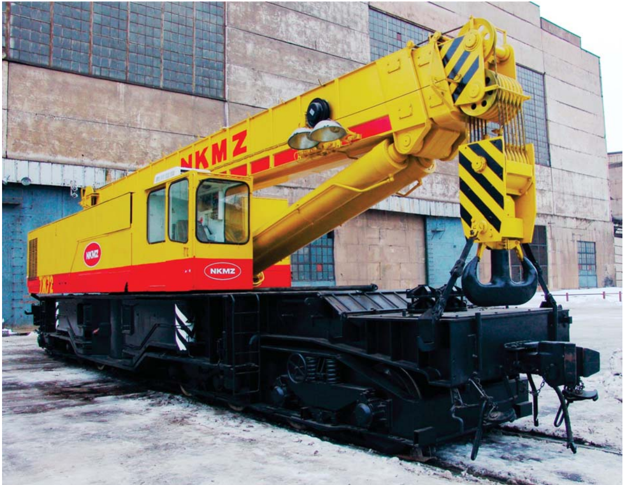
Self-propelled railway jib-type crane 7Ж72
