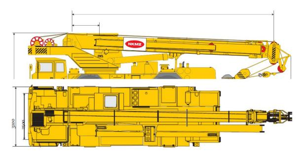
Jib design provides automatic extension of all jib sections, eliminating the presence of a "dead" segment.
