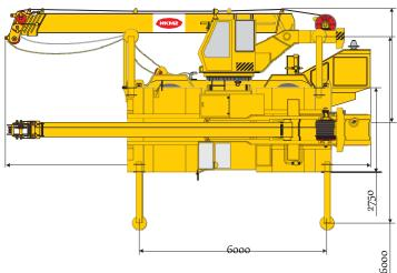
Self-propelled full-swing jib hydraulic crane KKS-30 with a lifting capacity of 30 t is designed for handling, construction and installation works while constructing buildings and structures, emergency recovery and installation works.
