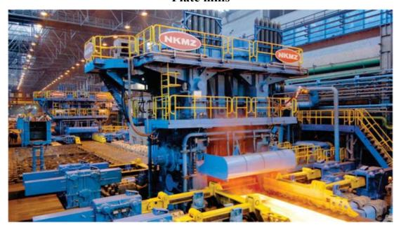
According to the Customer's request NKMZ produces equipment for plate mills ТЛС2000...5000 as complex and as separate machines.
