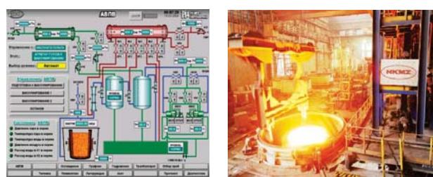
By means of VOD technology the high-chromium steel is obtained with the carbon content of <0,03%. The unified fleet of slide-gate ladles of the "Ladle-furnace" unit (having capacity 60, 90 tons) is used in order to effect steel vacuum degassing in the ladle (VD technology).
